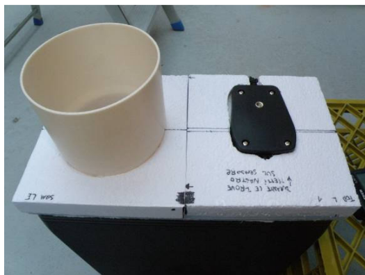
Figure 11: Calibration setup for SQM outdoor housing
