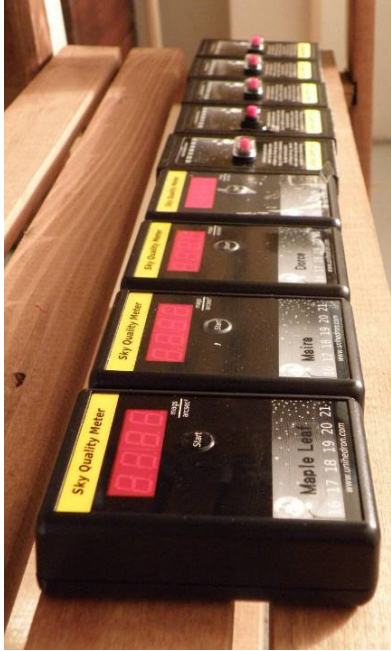
Figure 6: The nine SQMs subject to the cross-calibration.
